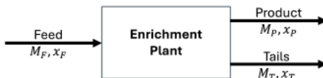
Figure 1. Material flow in an enrichment plant.
